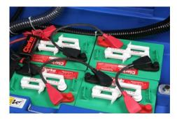
Easy access to the battery compartment is great for maintenance and installation and designed to contain any liquid spills. Choose either 242 or 310 Ah wet or 312 Ah maint-free (AGM) batteries.
