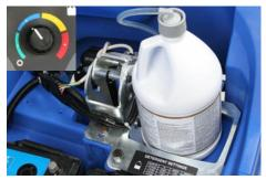
The optional Chemical Mixing System gauges the appropriate amount of chemical and mixes it into the solution flow. The ounce per gallon setting is controlled by a knob on the control panel.
